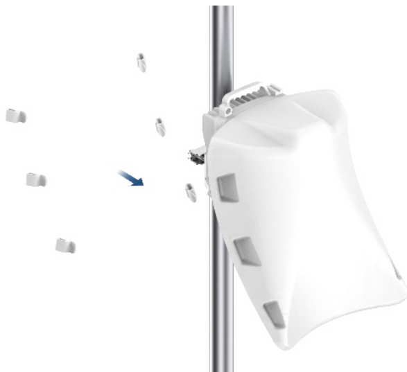
Align Radome to V3000 and attach with the supplied clips x 6
